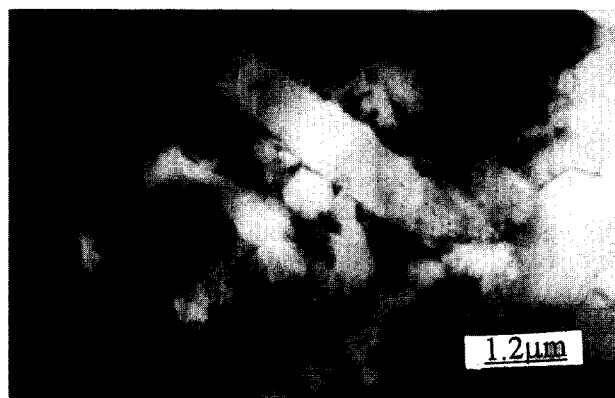
Fig. 1. Microstructure of GPS \alpha' - \beta' -Sialon showing equiaxed \alpha' -Sialon and elongated \beta' -Sialon grains.
